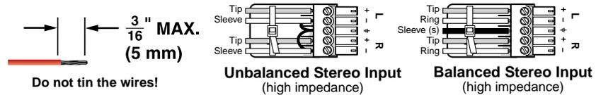
**Figure 2-6 — Captive screw connector wiring for inputs**
